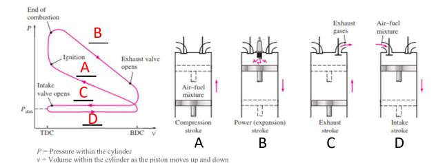
4. An actual four-stroke spark-ignition cycle curve (P-v curve) and description of the four strokes is shown above. For each arrow shown on the P-v curve, fill in the corresponding letter of the stroke.
