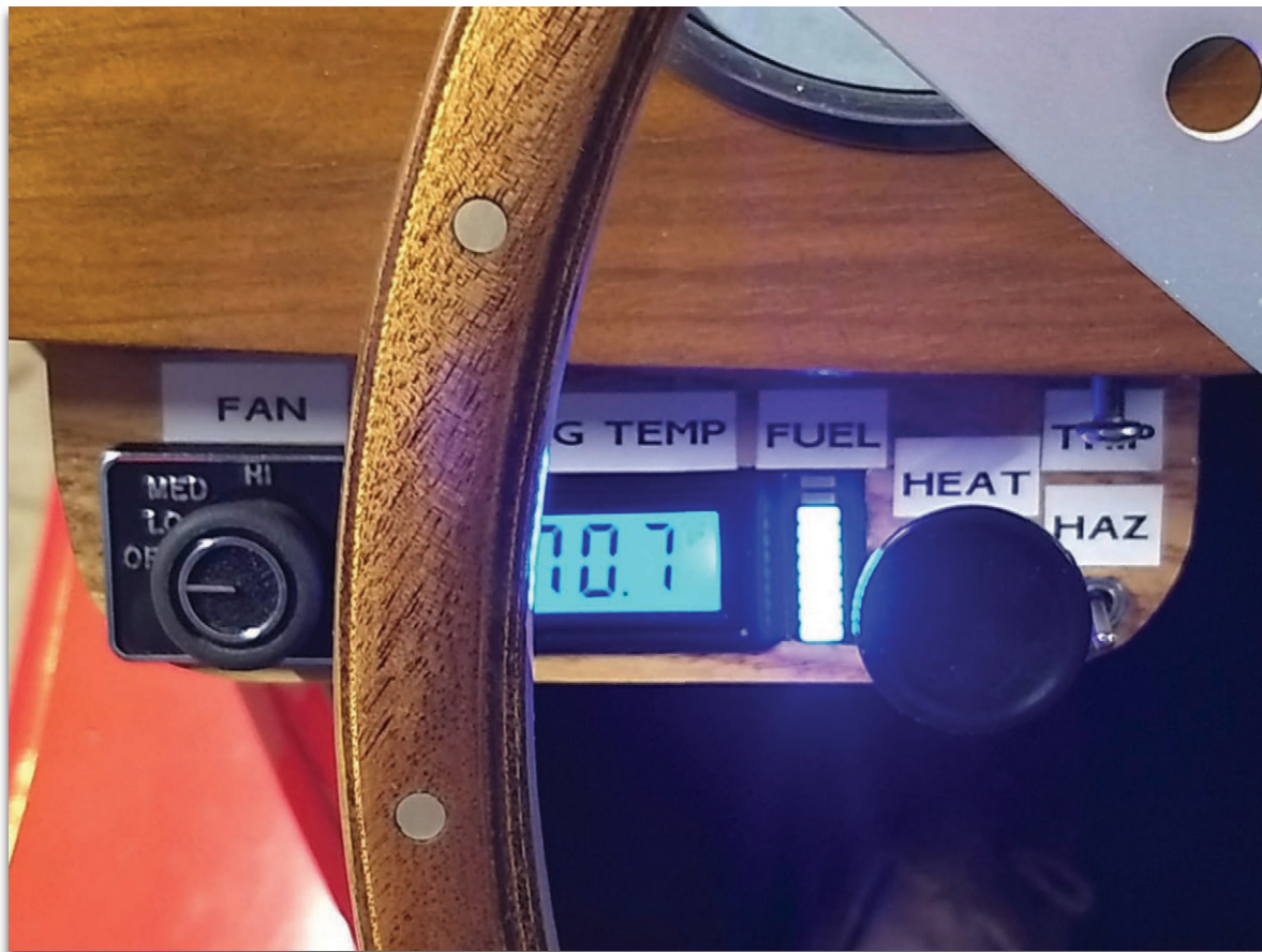
Discrete under dash controls and displays, including heater controls, temperature gauge, fuel gauge, hazard lights switch and trip odometer reset. Below: a full array of under dash fuses.
